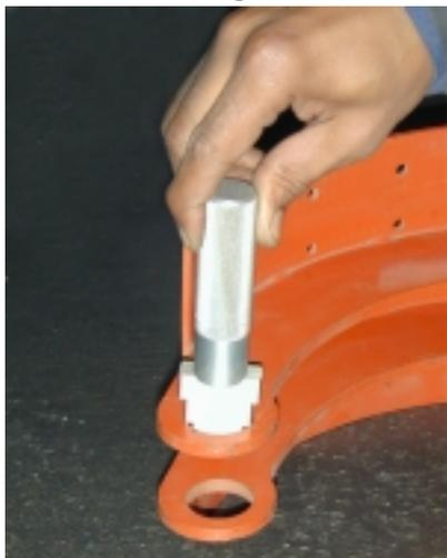
The camshaft bushing should be replaced at each normal reline interval. It takes up to one inch of push rod stroke to make up for forty-two thousandths of an inch clearance between the brake shoe and the brake drum. Proper replacement of the Cam Bushing will aid in Reduction of noise, Better Braking Efficiency and Proper Adjustment of Slack Adjuster.
