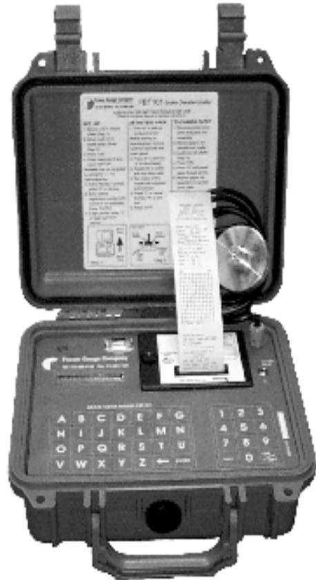
It is imperative that you maintain the decelerometers by regular maintenance and recalibration. Both the Tapley and the Fraser units should be recalibrated every two years to assure accuracy and acceptability in accident investigations.
