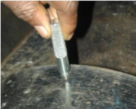
Shoes that exhibit bolt/rivet holes that have grown or been damaged in the removal of bolts/rivets should be scrapped. Use of shoes with large or distorted bolt/rivet holes can result in loose and cracked lining. Burrs or raised areas around the holes must be removed. Failure to do so may result in broken or cracked lining.
