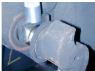
This gauge checks the Journal Area of the Camshaft for excessive wear and aids in the determination of proper replacement of the camshaft.
