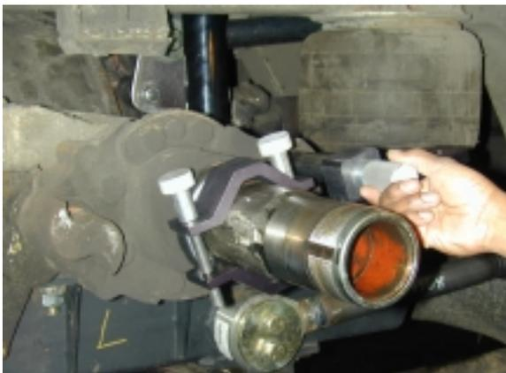
A spider gauge should always be used to check the alignment of the spider with the axle spindle. Bent spiders resulting from a frozen shoe or a seized pin cause the shoe to react slowly. Bent spiders should always be replaced. The proper fit will increase braking efficiency and reduce noise problems.
