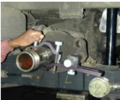
Brake shoe anchor pins should hold the shoe and lining assemblies parallel to the brake drum surface. If a brake spider or backing plate is bent or deformed in any manner, it, in effect, changes the relationship of the camshaft and anchor pin locations. Bent spiders cause partial lining-to-drum contact, resulting in erratic and noisy braking action and premature foundation brake component failure.
